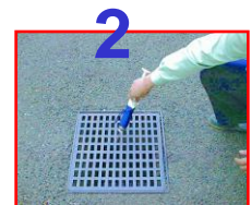
2 Pull handle of pump and take sample of gas
