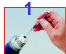
1 Connect detector tube to Kitagawa pump
